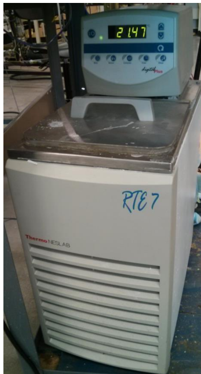
Figure 21. Test Stand Recirculating Chiller
